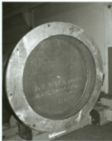
HSLA-100 Holding Bulkhead Panel Model: Before Test (Left) and After Hydrostatic Test to Rupture (Right)
